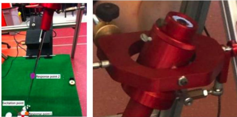
Figure 2. Left: Putter held in robot; Right: Robot clamping arrangement
